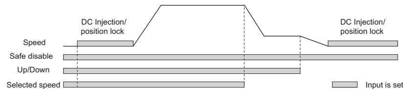
**Leveling Speed has Priority and the Leveling Speed Input is Assigned (d1-18 = 2, H1-□□ = 53)**
