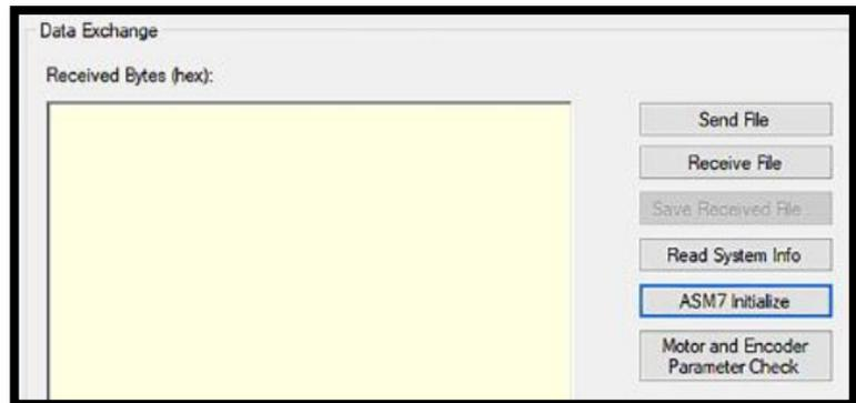
In order to delete the homing status, the serial number and an already existing container file in the ASM7, the “ASM7 Initialize” function must be locked by a password. For this the same principle as for the Digital Operator should be used. Means the password will be the last 4 digits of the ASM7 serial number.
